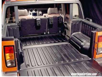
Figure 1.4 2005 General Motors Hummer H2 SUT's center bridge, sail panel, and box-rail protector [14]
